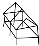
Post and Beam
